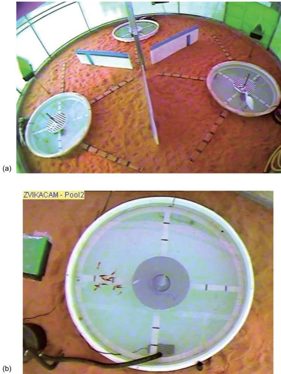
**Fig. 1.** (a) Panorama of the experimental arena as viewed from one of the digital cameras, showing the three equally spaced pools, each 0.76 m in radius. Note the egret in the pool on the right. (b) An experimental pool as viewed from above by its digital camera. The safe microhabitat is beneath the circular cover at the centre of the pool (radius 23.75 cm). Note the school of goldfish swimming to the left of the cover in the exposed/risky habitat.
