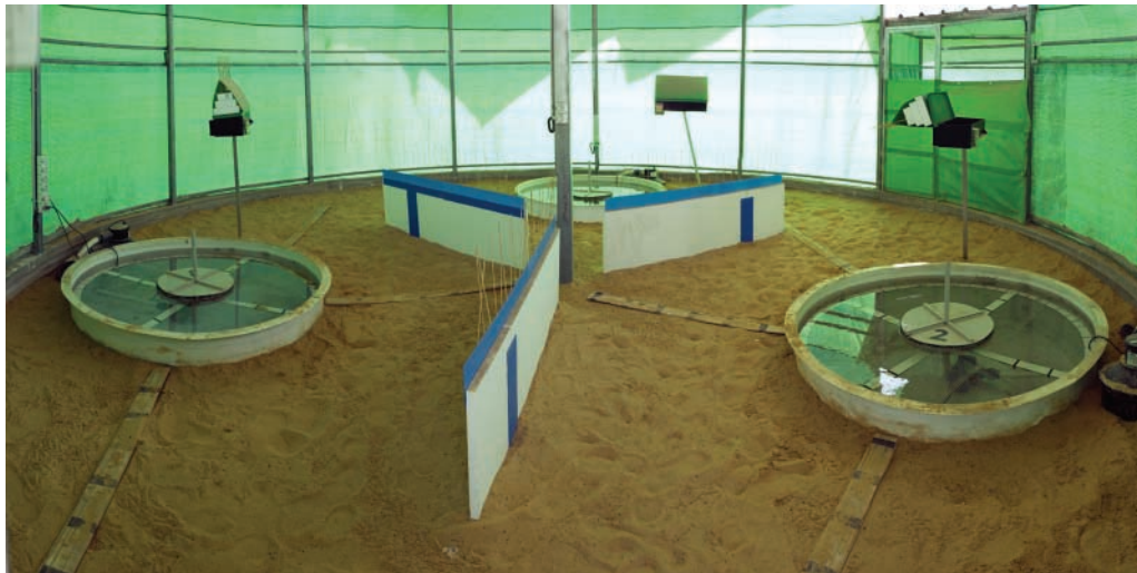
Fig. 1. Panoramic view of the experimental arena. There are three equally spaced pools, each 0.76 m in radius. In the centre of each is a disk (radius 23.75 cm), which fish can hide under. Each pool has its own pump (not seen), feeder, and filter. To prevent egrets from seeing more than one pool at a time, we installed opaque partitions. We put vertical wooden skewers on all partitions and feeders to prevent the birds from perching atop them.
