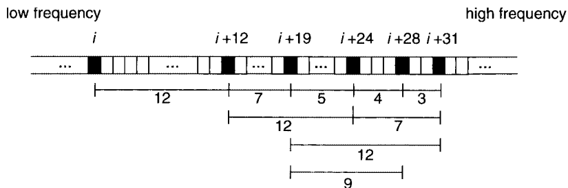
Fig. 2. Intervals between harmonics accompanying a single basic tone. i indicates the fundamental; the other black squares represent the harmonic tones. The numerals indicate the length of intervals, given as the number of semitones included. These intervals are all consonances.
